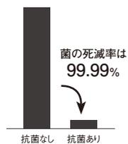
We added an antibacterial function to the ceramic glaze to meet the needs of the times. Silver has long been used as an antimicrobial agent. Applying a silver-based antibacterial coating on the surface of the glaze, the effect is long and stable. The target bacteria are Staphylococcus aureus and Escherichia coli, which have the effect of suppressing the growth of the bacterial on the ceramic surface.
